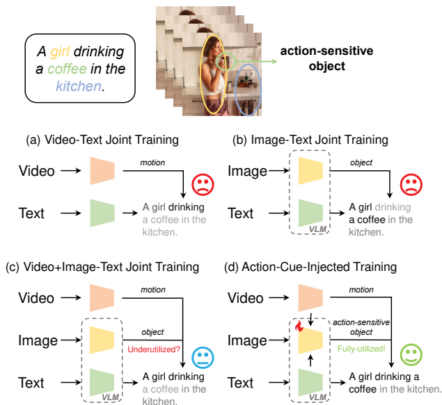
Figure 1: Illustration of feature extraction pipelines. The image encoder in VLM can capture more detailed features of static objects, but may not be able to distinguish action-sensitive objects from backgrounds. Action cues from other modalities are necessary to guide the image encoder in recognizing action-sensitive objects, making it fully utilized.
